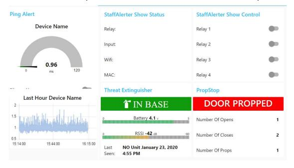
PropStop is a Wi-Fi connected, battery powered device that mounts to any door. Information on the door position is sent to the StaffAlerter Dashboard for status. A time value is set to determine what period a door is left open before the system determines a propped open condition exists.
