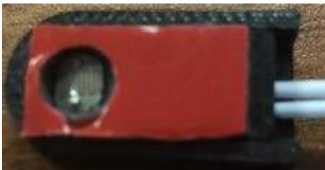
Light Sensor with Adhesive Backing
